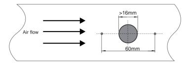
The arrow engraved on the sensing head of HWS indicates the direction of the air stream during factory adjustment. When installing the HWS probe, make sure that the arrow matches exactly the flow direction.
