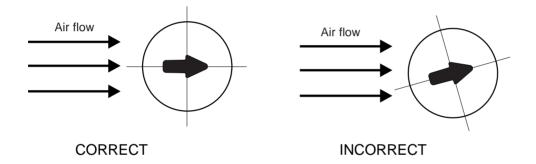
The mounting flange allows for precise setting of the HWS immersion depth in a duct. The entire sensing head must be in the air flow to be measured.
